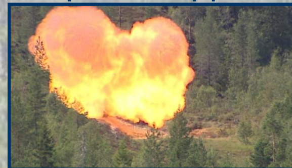
The worlds first full scale burst test of hydrogen pressurized pipeline
