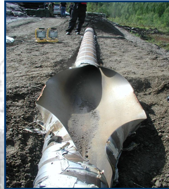
The worlds first full scale burst test of hydrogen pressurized pipeline
